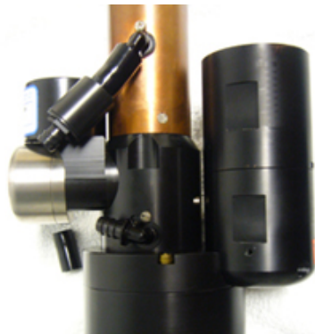
Figure 14 Exhaust tube removed from elbow fitting
